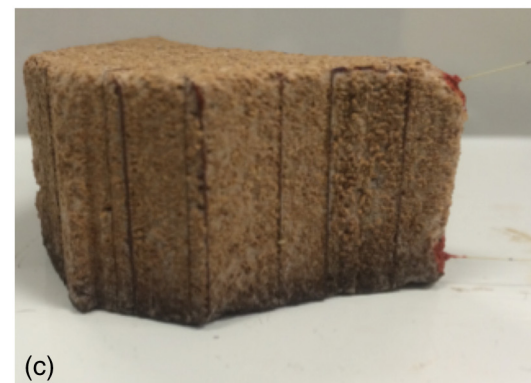
Fig. 12 SLA sample: (a) IR image at point of maximum temperature in test 1-2, (b) before and (c) after test 2-1 described below.
